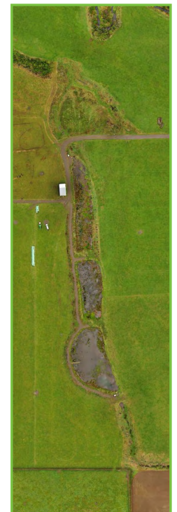
Newly constructed and planted wetland (left) showing direction of flow through initial deep sedimentation pond and subsequent two shallow elongated cells. Plant cover after one year shown on the right.
