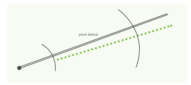
• Put half of the buckets in the first 2/3 of the pivot (closest to the pivot point) and half in the last third.
