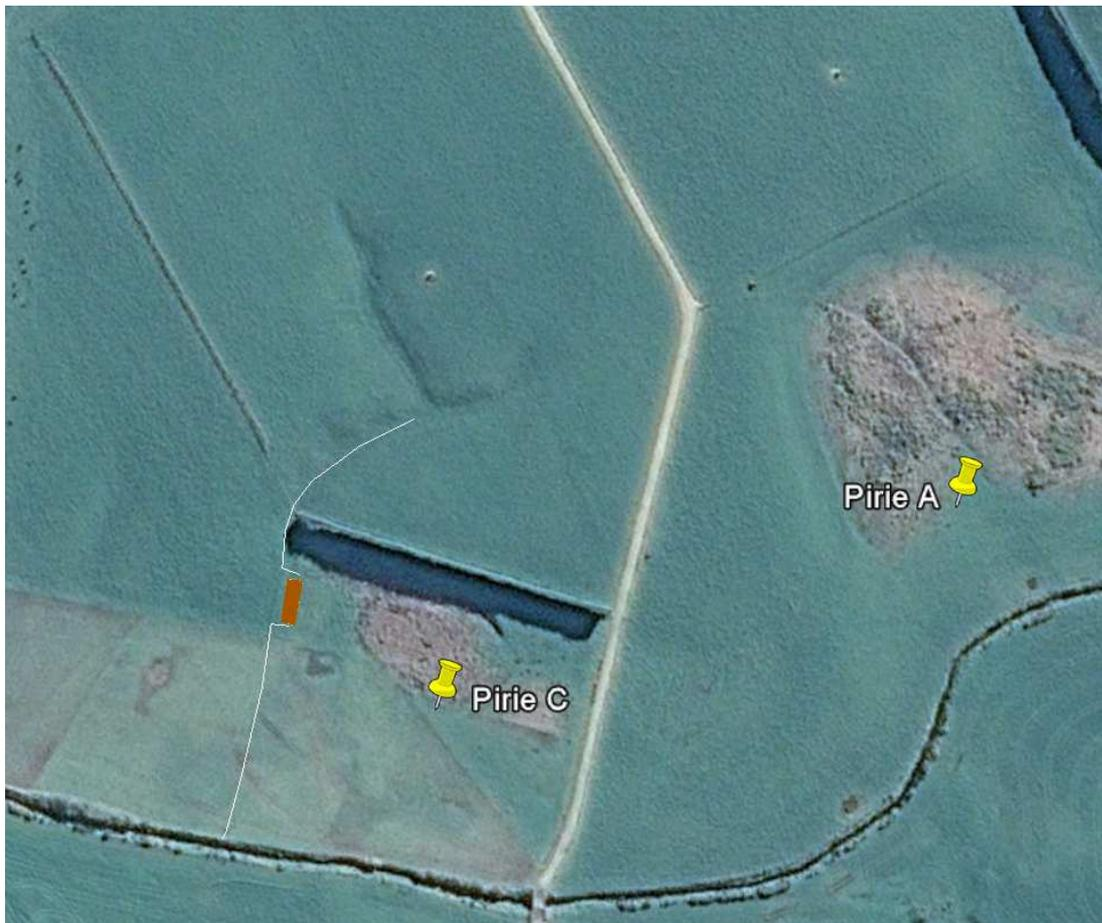
**Figure B-4: Potential site for wood-chip filter on Pirie Farm.** Subsurface drain flow to be diverted via weir into filter and then returned to drain at exit. High flow bypass via drain to be maintained.
