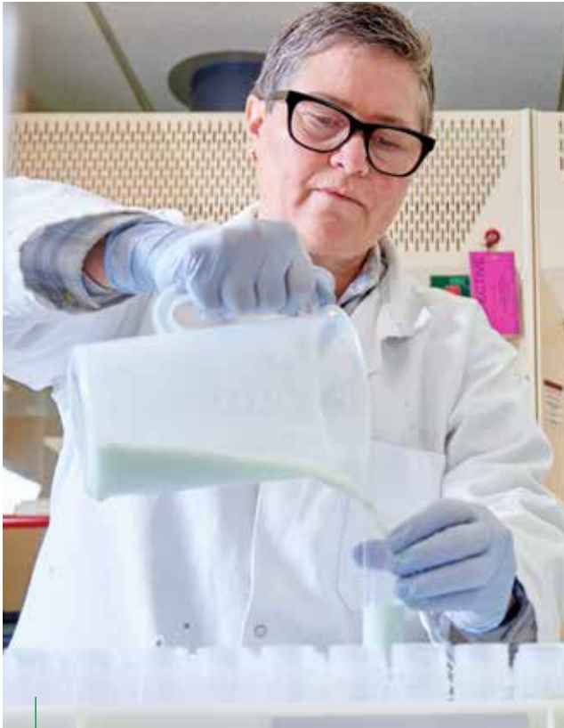
Tash Leach, DairyNZ senior research technician, testing pilot and calibration samples with milk which contains Bronopol, a preservative to prevent microbial growth, and methyl blue dye as an indicator.
