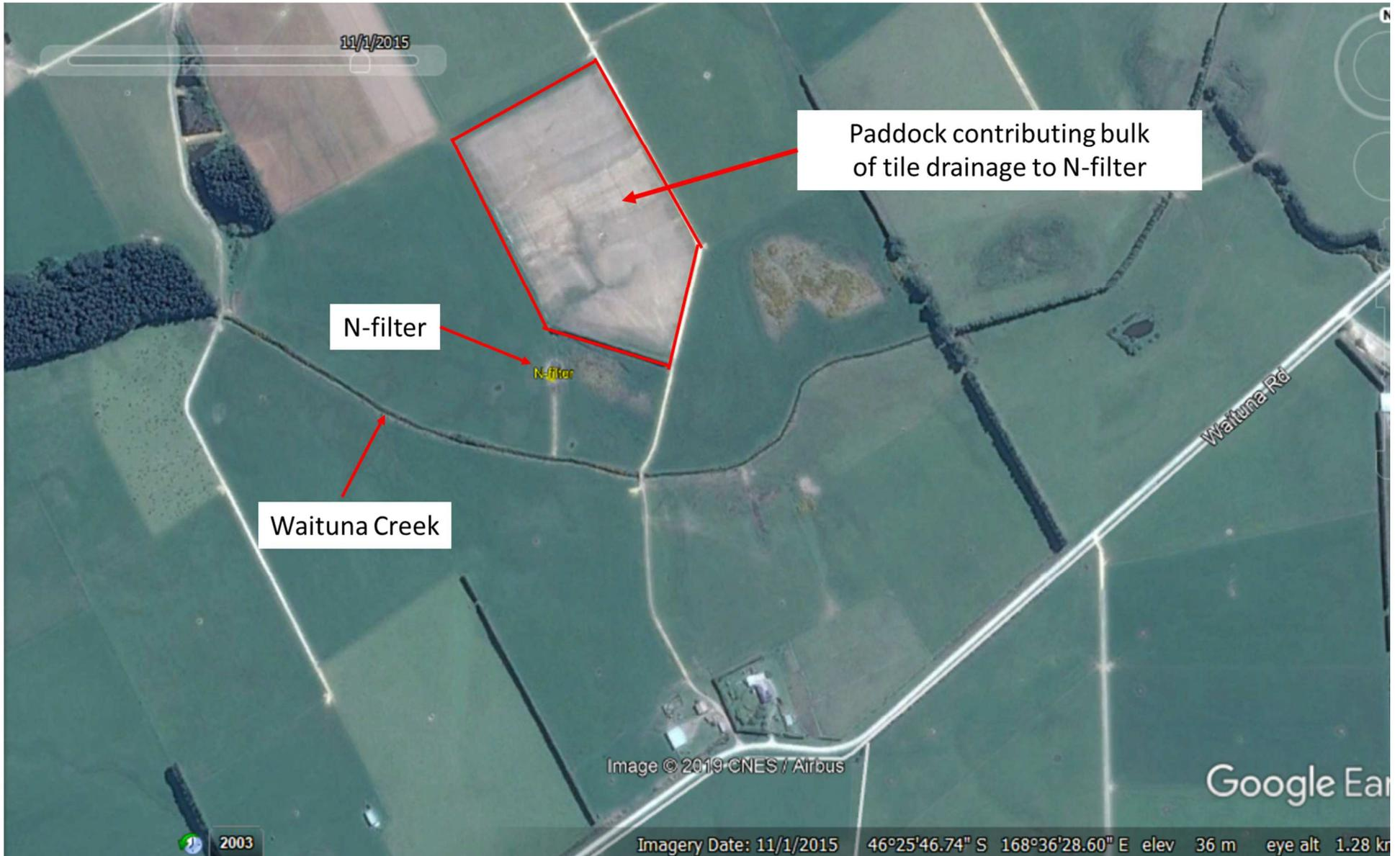
Figure 2-2: Location of nitrate-N filter relative to the paddock which is the principal source of shallow groundwater draining into the filter. Waituna Creek flows from right to left.
