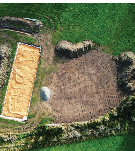
Balfour dairy farmer Brendon Stevens now has a wetland and bioreactor as part of the Balfour Catchment Group project using science solutions to reduce nitrogen loss.
