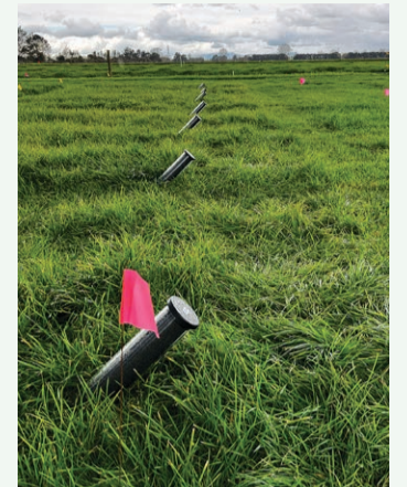
A rhizotron installed in the research plot. The transparent tube lets researchers lower a specialised camera into the soil to capture high-resolution images of plant roots.
