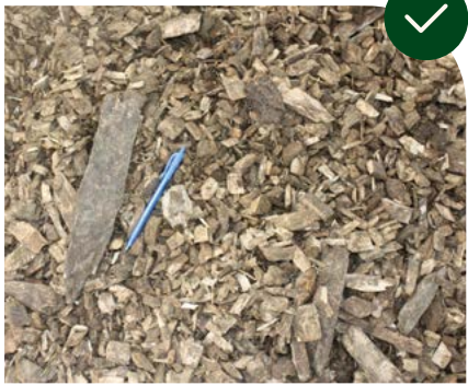
Use pine or a timber type that chips square and not stringy.
