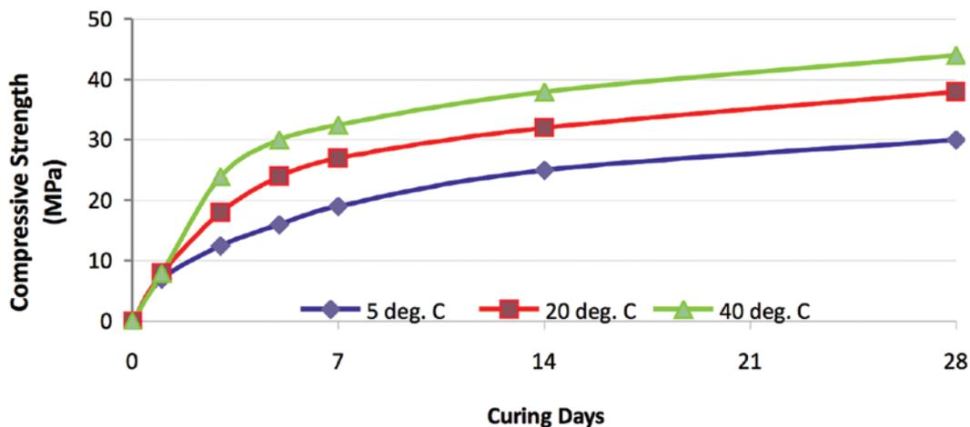
Proper curing through moisture and temperature control is essential to ensure the required durability and strength is achieved, and is particularly important for surface durability.
