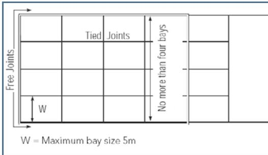
Figure 4: Joint spacing
