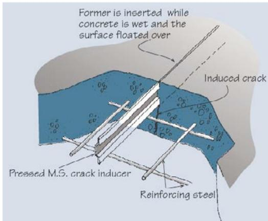
**Figure 19:** Crack inducer (for reinforced or unreinforced slabs)
