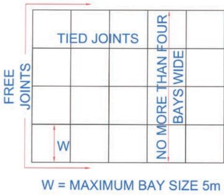
For slabs that are not categorised as having to meet the Building Code and where reinforcement is omitted, joint spacing (free joint) should be reduced to 3 m intervals.
