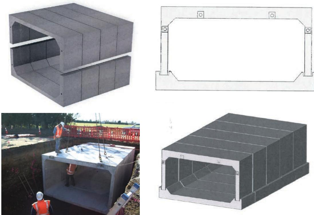
Box culverts can be specifically designed to provide the required foundation strength under the road pavement. As the internal base of the box is the floor of the underpass, boxes provide some construction savings by eliminating the need to pour an *in situ* base. Interconnecting precast wingwalls and headwalls are available. Starter bars can be cast into end units so as to tie into *in situ* poured wingwalls or apron floor slabs. Various joint sealing options are available.
