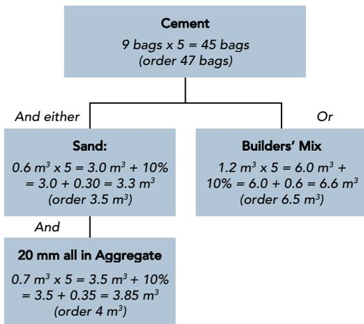
For proprietary pre-bagged concrete, the bag and instructions will indicate the approximate yield per bag. Allow for at least one extra bag in case a bag is damaged. Use the same product for the whole job.
