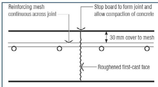
Figure 8: Construction joint
