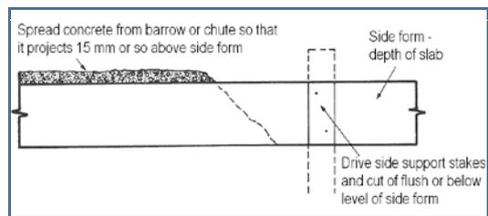
**Figure 9:** Placing Concrete
