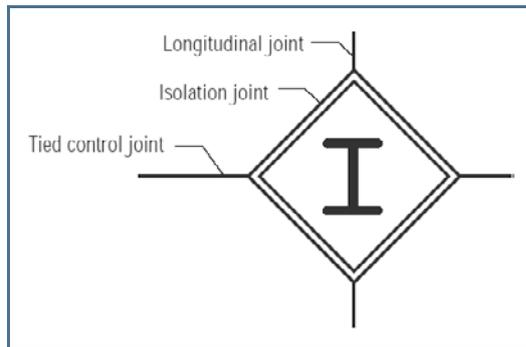
Figure 7: Isolation joint
